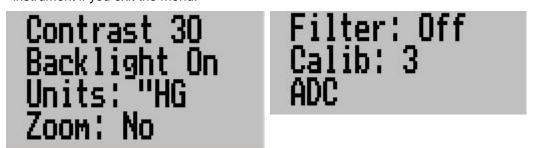
Technical setup functions "Calib" and "ADC": (accessible only if you start up the instrument while pressing both "+" and "-" buttons at the same time)
