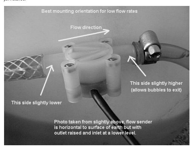
For installations were long fuel lines are unavoidable we recommend to fit the fuel flow sender AFTER the fuel pump. Install a second fuel filter before the sender to act as reservoir to prevent pressure pulses from the fuel pump to affect the fuel flow reading accuracy.
