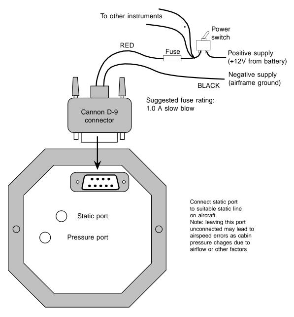
Connect the pressure port to a pitot tube. The location of the pitot tube should be choosen so it is exposed to clean, undisturbed airflow at the same speed as the aircraft if flying.
