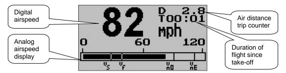
To view the flight log, use the relevant Menu function as described below. The ASI-3 uses the following algorithm to determine if a flight is in progress:
