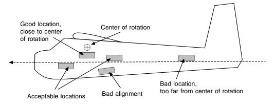
The drawing also gives an example of a bad alignment. Please try and locate the IMU such that it is aligned with the aircrafts axis of travel at cruise power setting.
