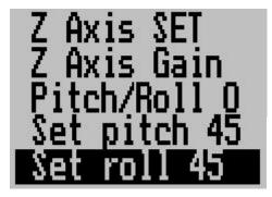
Functions Set North, Z Axis SET, Z Axis Gain, Pitch/Roll 0, Set Pitch 45, Set Roll 45 are technical functions that are accessible only in technical mode. To enter this mode, start the A/C-1 (switch on power) and wait until you see the introduction display. Then press both + and – keys at the same time. The A/C-1 will continue operating normally but will show the additional technical setup/calibration functions as shown.
