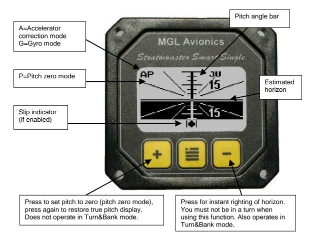
In order to correct the horizon display, you need to fly straight and level. The horizon will correct itself in this case given some time (about 15 seconds to a minute depending on severity of the error). You can also press the "-" key to force an immediate correction. You must fly straight and level for this to work correctly.
