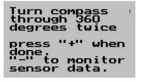
Proceed as instructed and turn the aircraft through a full 360 degrees at least once. Allow this procedure to take some time, perhaps a minute. You can proceed to turn your aircraft though two or even more turns but you need to fully complete at least one turn.
