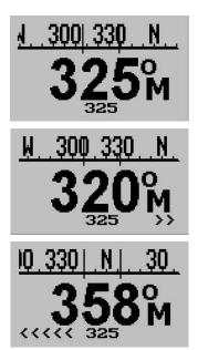
"+" pressed at a heading of 325 degrees. Currently the heading equals the course to steer as shown below the heading. No steering indicators show.
