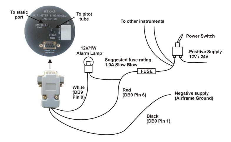
The use of an external 1A fuse is recommended. Connect the supply terminals to your aircrafts power supply. The ASI-1 can be used on both 12V and 24V without the use of any pre-regulators. Ensure that the supply voltage will not drop below 8V during operation as this may result in incorrect voltage and or current readings.
