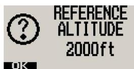
Enter the reference altitude you would like to use in relative mode. Use the rotary control to adjust the reference altitude. Press the F1/up key to accept.
