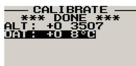
The ALT-4 is calibrated in degrees Celsius. The ALT-4 is calibrated at the factory using a precision laboratory thermometer. If recalibration is required then adjust the value using the up/down keys or the rotary control until the temperature matches the reference ambient temperature.
