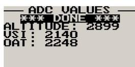
This menu displays the ADC values that have been read from the pressure sensors.
