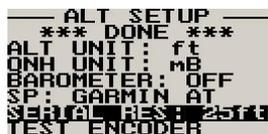
Select the resolution of the output data, a selection of 1,10,25 or 100 ft can be made.
