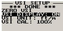
Select if you want to show the built in VSI (vertical speed indicator). The built in VSI will be shown above the altitude readout.
