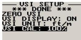
This is a function that is used to calibrate your VSI to read exact rates of climb or decent. This function works as a percentage of initial reading. The default setting for this function is 100%. Increasing this value increases the VSI reading and decreasing the value decreases the reading.
