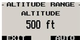
The installer can put the ALT-4 into an auto test mode or a manual test mode. The auto mode will increment the altitude at 100ft per second from -1200 to 30000. In the manual mode the installer can rotate the rotary control to a desired altitude. Press the F1/Up key to exit the test.
