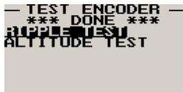
The ripple test is for the parallel Gillham output only. This test will continuously loop and assert one line at a time starting at the C4 output line and ending in the D4 output line. This test is handy to see if all lines are correctly connected from the ALT-4 to the transponder.
