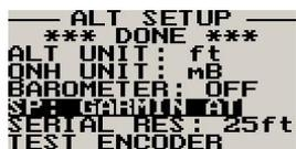
Select the protocol of the RS232 output message. The protocol can be selected between GARMIN AT, Magellan, Northstar/Garmin, Trimble/Garmin, MGL Avionics and Microair UAV. Please see section 5 for more information.
