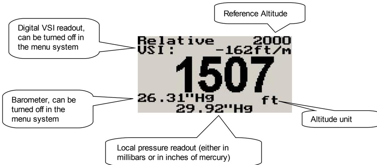
Use the rotary control to adjust the local pressure setting. Pressing the F1/up key will allow the pilot to enter a reference altitude.
