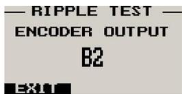
The line that is currently asserted is displayed on the screen. Press the F1/Up key to exit the test.
