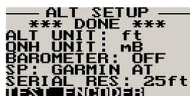
This is a handy function to test the ALT-4 transponder interface once installation has been completed.
