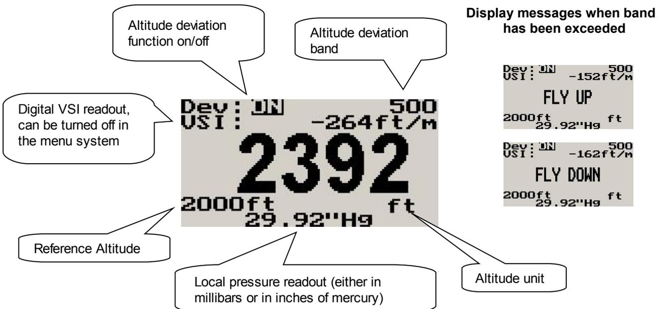
Use the rotary control to adjust the local pressure setting. Pressing the F1/up key will allow the pilot to enter a reference altitude and the deviation band.
