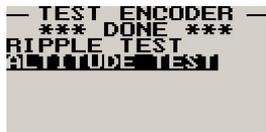
The altitude test can be used to test both the Serial as well as the parallel Gillham output. The altitude test allows the installer to key in a desired altitude and to see if the transponder altitude corresponds.
