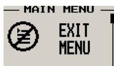
Pressing the rotary control on this menu item will cause the ASX-1 to exit the menu system. All changes made during navigation of menu system will be saved in non-volatile memory on exiting the menu system. If you remove power before exiting the menu the instrument will not save any changes.
