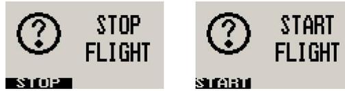
Press the F1 key during the normal display mode to manually start/stop a flight. This key is only active if the ASX-1 is setup to select the manual flight option under the log book setup menu.
