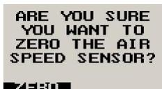
This setup allows your instrument to measure the zero airspeed reading of the airspeed sensor and set a calibration value internally for this. This is equivalent to some mechanical airspeed indicators that have an adjustment to set the needle to zero when the aircraft is not moving. You would use this function occasionally if you see an airspeed reading when the aircraft is at rest. This
