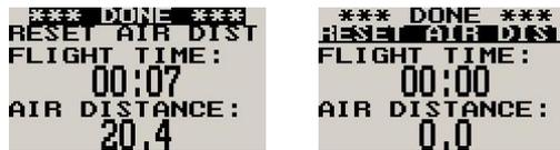
**Note:** The air distance trip counter measures distance flown through the air. This is not the same as distance flown over the ground unless you are flying at sea level at zero wind speed. The air distance shown is subject to under reading at altitude due to decreased air density.
