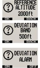
Adjust the reference altitude using the rotary control. This is the altitude that the pilot wants to maintain. Press the F1 key to accept, press the F2 key to return to the main display.
