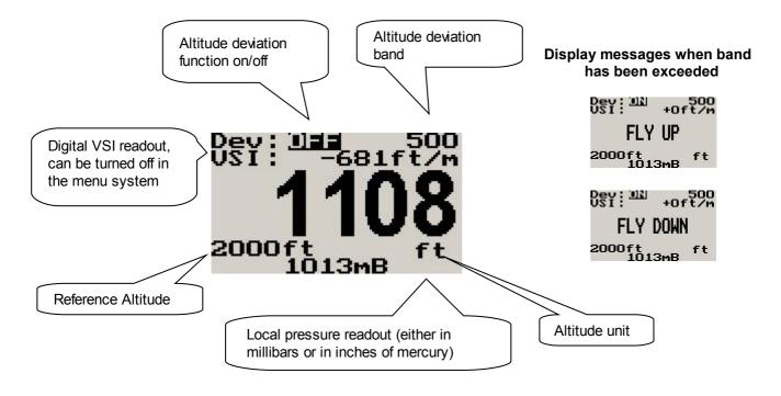
Use the rotary control to adjust the local pressure setting. Pressing the F1/up key will allow the pilot to enter a reference altitude and the deviation band.
