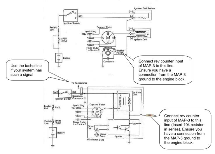
Electronic ignition system with conventional ignition coil
