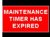
This function allows you to set an engine maintenance timer. This timer is set in engine hours and it will count down to zero when the engine RPM is greater then the "HOBBS RPM". A good use for this function is to set the hours until your next spark plug change or engine inspection. Use the rotary control to change the value.
