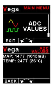
This menu displays the ADC values that have been read from the pressure and temperature sensor.
