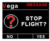
Press the F1/Up button during the normal display mode to manually start/stop a flight. This key is only active if the MAP-3 is setup to select the manual flight option under the "TIMERS" setup menu.
