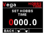
This function allows you to set the engine Hobbs meter to any value. Typically, you would use this function to set the Hobbs meter to the current known engine time. Use the rotary control to change the value. Press the rotary control to accept and exit the menu option. If the Hobbs code is set to another value beside zero, then the pilot will be prompted to enter the Hobbs access code before allowing him to change the Hobbs time. This feature is useful for charted and flying school planes.
