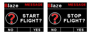
Press the F1/Up button during the normal display mode to manually start/stop a flight. This key is only active if the MAP-4 is setup to select the manual flight option under the "TIMERS" setup menu.
