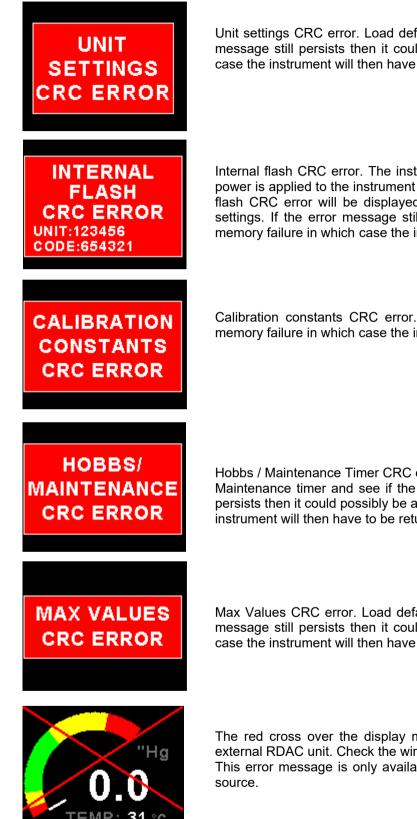
Unit settings CRC error. Load default settings to restore to factory defaults. If the error message still persists then it could possibly be a non-volatile memory failure in which case the instrument will then have to be returned to the factory.
