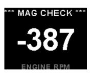
Press the F2/Down button once you have reached your normal run-up RPM. The display will show the RPM deviation from when the magneto function was activated. Any RPM drops will be displayed as a negative RPM value, a positive reading indicates an increase in RPM.
