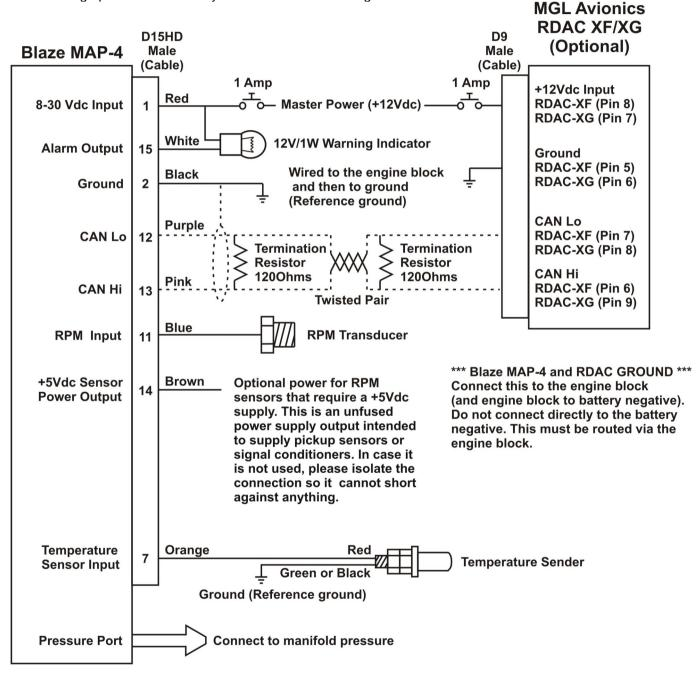
**Please note:** The +5V Sensor power output line is unprotected and intended only for the supply of a hall-effect, optical or gear tooth sensors. Connecting any voltages (such as the 12V supply) to this line could destroy the instrument. The +5V line may supply currents of up to 50mA. Should your sensor require greater currents you must supply it from another source.
