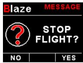
Press the F1/Up button during the normal display mode to manually start/stop a flight. This key is only active if the ASI-5 is setup to select the manual flight option under the "TIMERS" setup menu.
