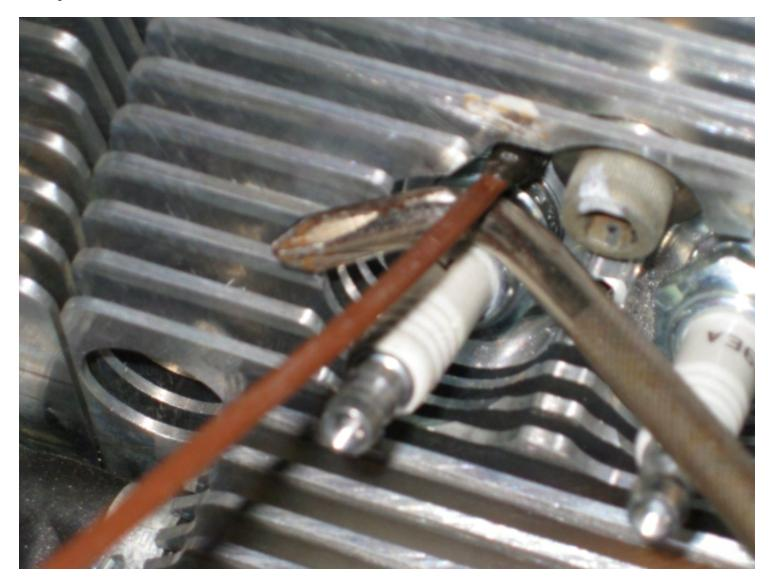
The expoxy in and around the crimp barrel is the most brittle and fragile part of the sensor assembly, but the hard, relatively inflexible wire is also very vulnerable to tight or repeated bending, and should not be bent to a smaller radius than is absolutely necessary.
