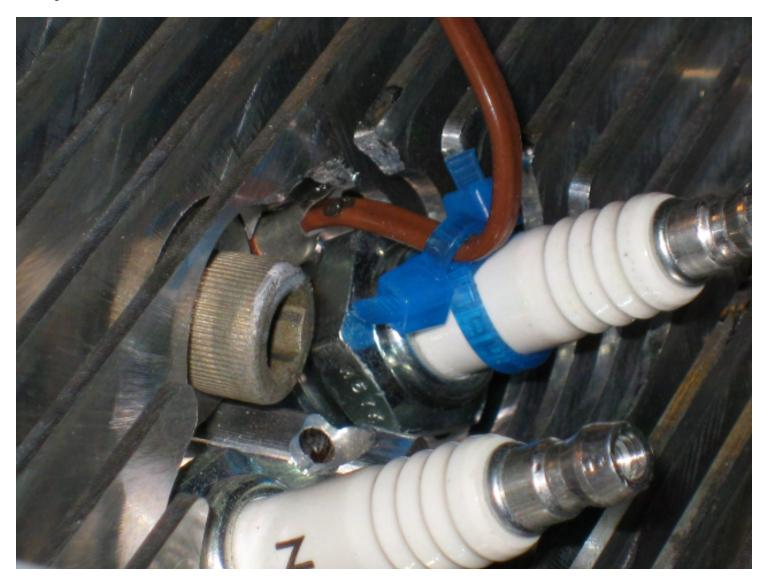
The double tie wraps secure the wire from further bending at the top of the sensor epoxy, and will hold the wire off the plug slighty, for slightly better cooling and some chafe protection. In the photo above, you can also see how the wire <u>has</u> pulled away (separated from) the original, gray epoxy. It also shows an imperfect early attempt to add **JB Weld** epoxy at the top of the crimp barrel. If it's not too bad, this can be fixed in place, by carefully adding more epoxy.
