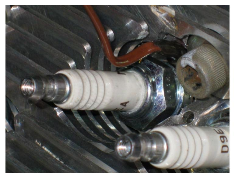
The next photo shows how the wire is secured to the plug with double, high temp Tefzel tie wraps. These are the small 4" long ones available from <u>Steinair</u>, among other sources. (This photo is taken from a different cylinder, on the left side of the engine. The rear of the engine is toward the upper right.)
