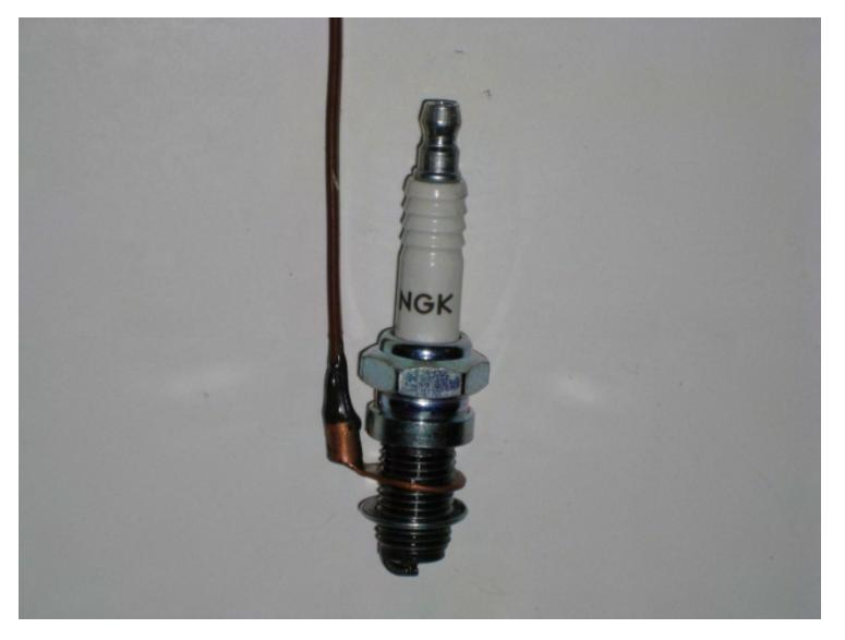
In the photo above, you can also see how the sensor crimp barrel has been slightly bent out, so it will lean away from the top of the plug.
