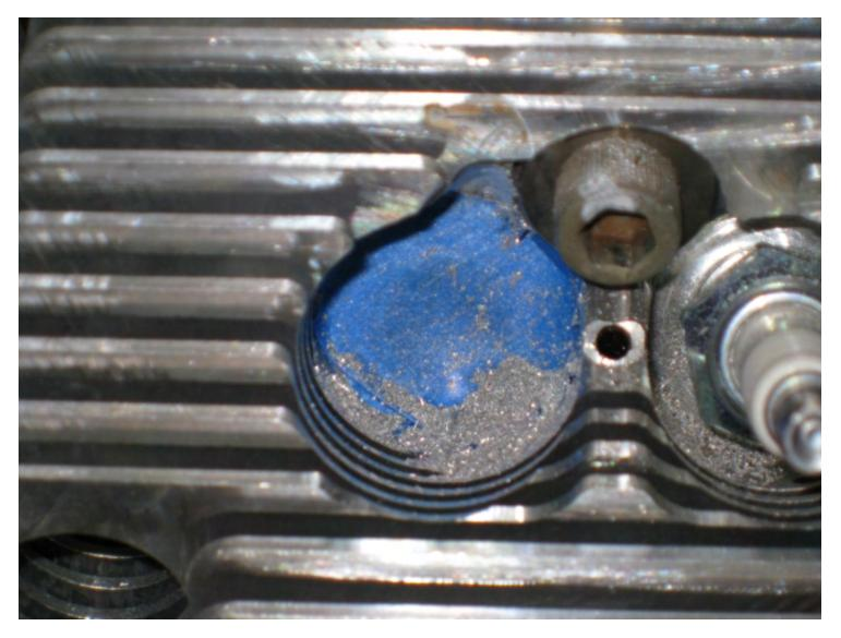
In the photo above, the "butte" is gone and the excavation has begun to go down the side of the vertical, cylindrical wall -- but the tape is still in the way. Gotta get that squished down some more. Again, the small, dark hole between the taped hole and the second plug on the right isn't covered up. It should be.
