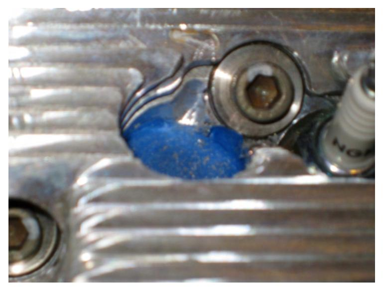
Time to install the CHT sensor and plug. Just a reminder, the sensor screws onto the plug threads first, then the plug washer goes back on, like this:
