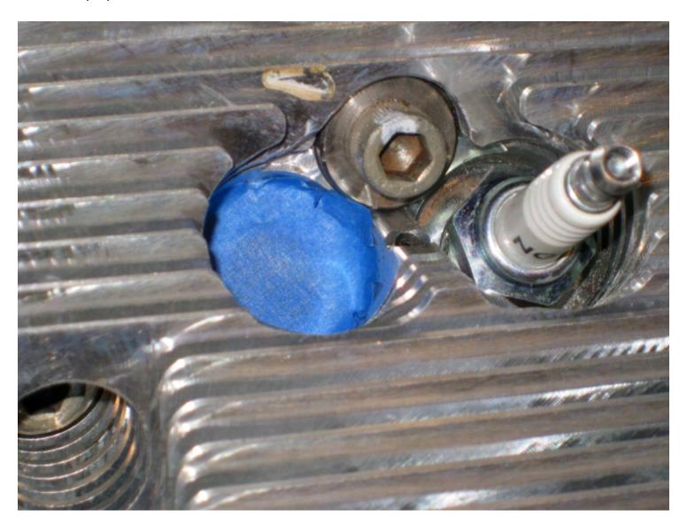
Obviously, we have to keep metal filings from falling into the cylinder, so the hole is covered with tape. (Unlike standard sand colored masking tape, the blue painter's masking tape will not leave residue.) You may need to use a Q-Tip swab to clean oil or whatnot off the plug washer seat first, so the tape will stick. A Q-Tip that is just barely damp with acetone or MEK will do the job. (You don't want to be sending drops of those chemicals down into the cylinder either!)
