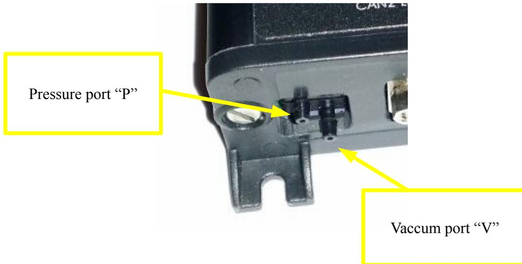
The sensor ports are suitable for 2mm inside diameter PVC tubing or similar. **Please do not exert any large force while working with these ports.** They can break and excessive force can also break the sensor off the internal PCB.
