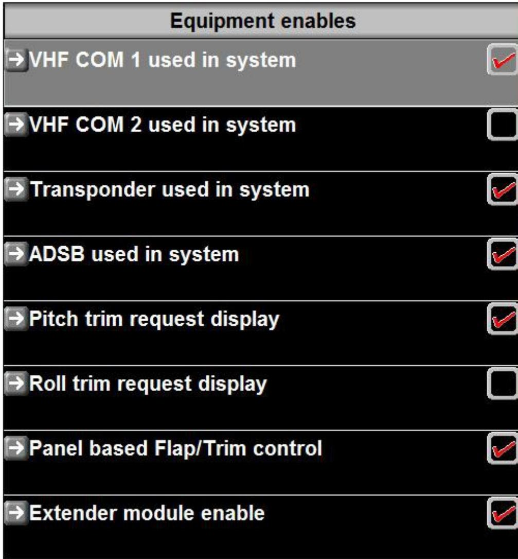
Once connected, please enable the Extender module in the Equipment Enables menu (this is in the System Setup menu). You need to restart (power cycle your EFIS) to complete the installation. Please save your new setting by exiting the menu in the normal manner before removing power.
