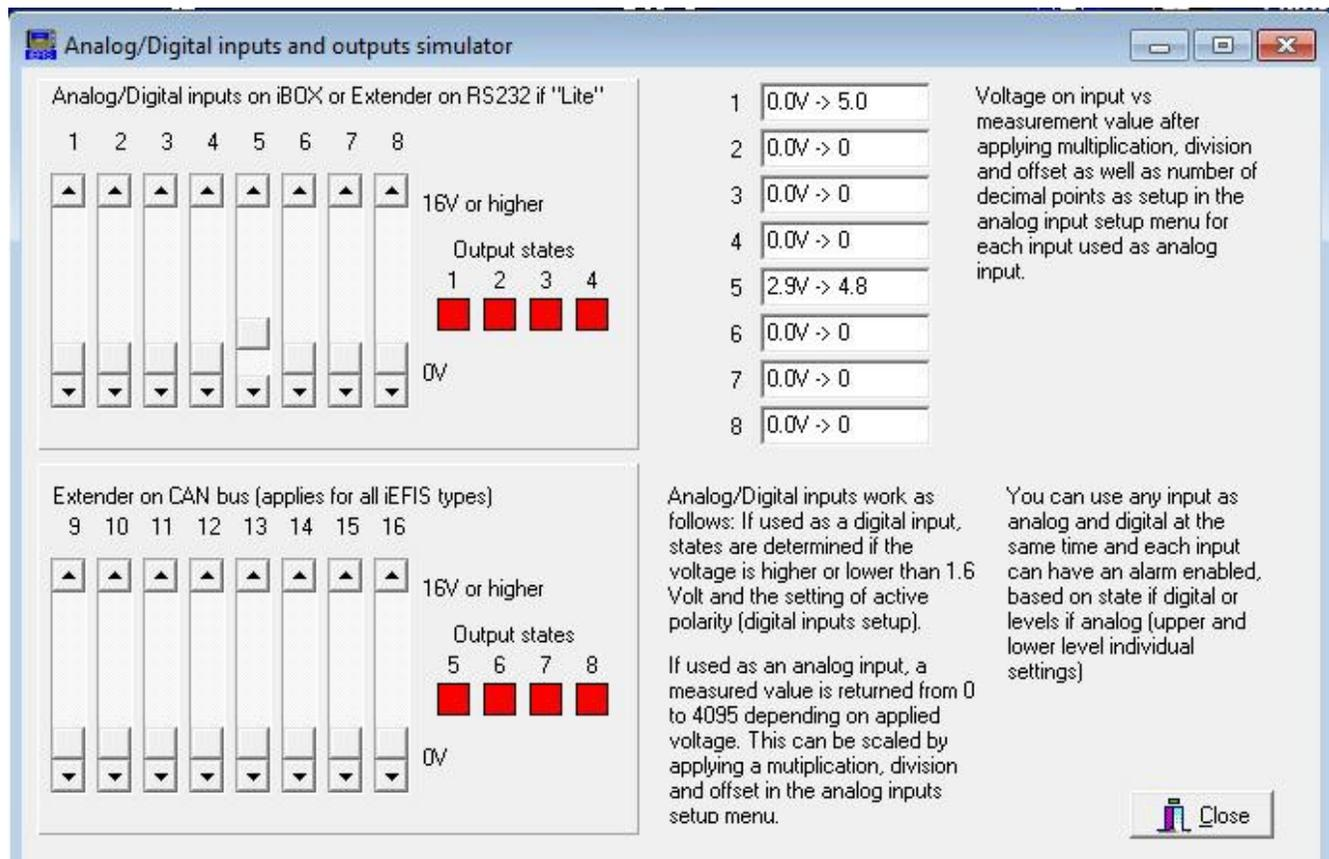
The iEFIS screen designer and simulator contains a useful tool that allows you to simulate the analog inputs as well as the outputs.
