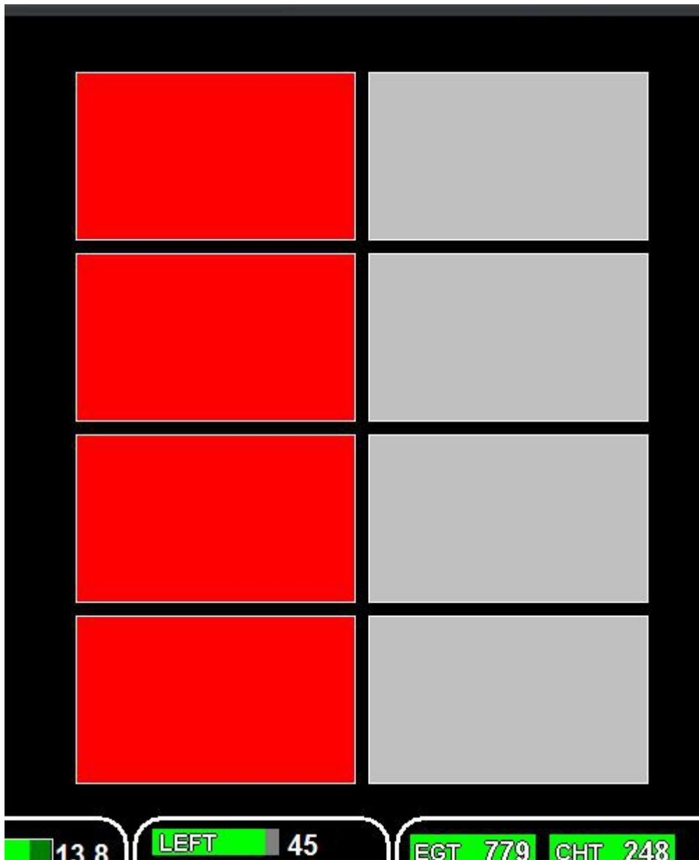
Basic example of a screen design including 8 touch fields connected to digital outputs. You use the “touch field” component, set it to an output function (ON, OFF or TOGGLE) and then select “visual” and give it desired colors for the ON and OFF states. You can also just show them as “states” in which case touching them will not change their state.
