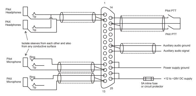
This diagram shows a typical two place setup for a pilot and single passenger for two headsets.
