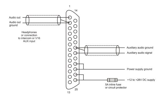
The audio output may be wired to a headset, speaker or an audio input of a suitable intercom. It may also be wired to the AUX input of a V16 transceiver to form a combined NAV/COM. In this case the AUX input of the N16 becomes the AUX input of the combined NAV/COM system.
