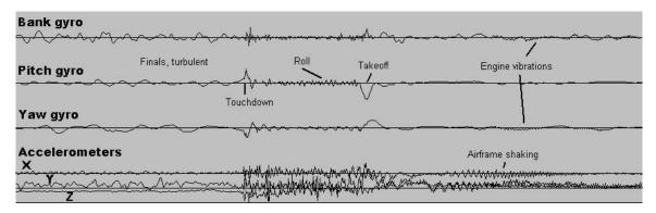
The SP-3 was installed on a ultralight aircraft, no provision was made to dampen any engine or airframe vibrations. The SP-3 was simply taped to one of the airframe members. The resulting horizon display was correct thoughout the flight. This serves to give an indication of the abilities of the SP-3 firmware.
