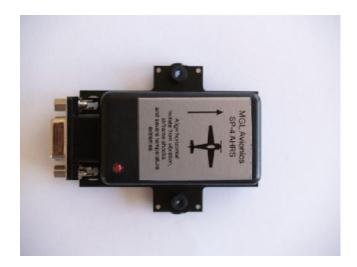
The SP-4 AHRS is MGL Avionics's fourth generation AHRS system. It is also the smallest and lightest, yet it packs an incredible system:
