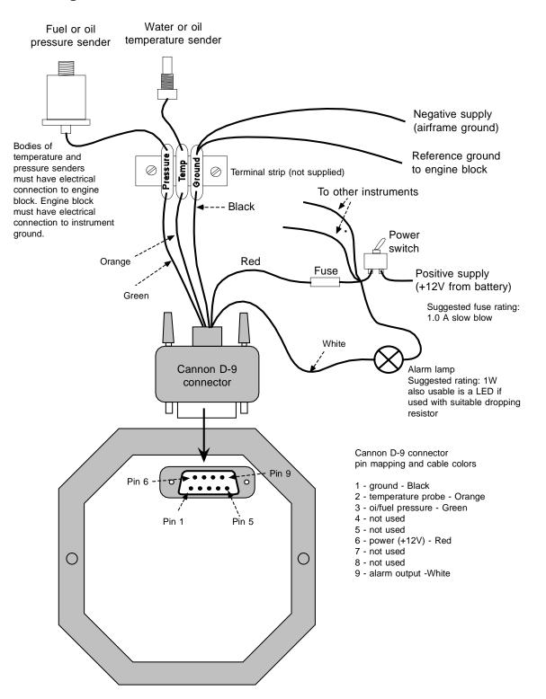
Connect the supply terminals to your aircraft's power supply (you need a dropping resistor or preregulator for 24/28V systems).
