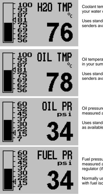
Coolant temperature, usually water temperature of your water cooled engine.
