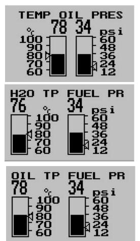
Combined oil temperature and oil pressure display. Most oil sump or dry sump lubricated engines require monitoring of both oil temperature and oil pressure making this option very valuable.
