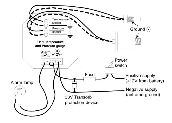
Connect the supply terminals to your aircraft's power supply (you need a dropping resistor or preregulator for 24/28V systems).
