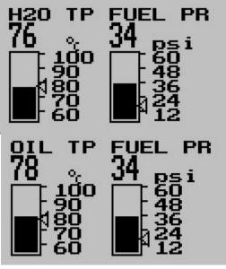
Combined coolant temperature and fuel pressure display. A suitable choice for many water cooled engines.
