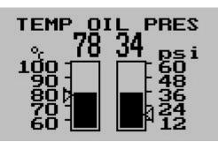
Combined oil temperature and oil pressure display. Most oil sump or dry sump lubricated engines require monitoring of both oil temperature and oil pressure making this option very valuable.
