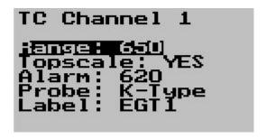
Selecting to setup any of the four channels results in a display similar to the above. When you have finished with your setup, press the Menu key to exit.
