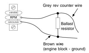
Note: On Rotax DCDI ignition systems it may be required to install a ballast resistor as shown. A typical value is 220 ohms. Many installations can omit this.
