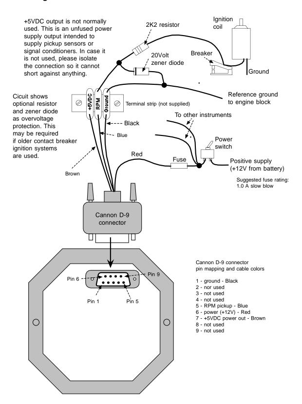
Installation of the RV-3 is quite straight forward in most cases. The above drawing shows a typical connection for a standard "old fashioned" contact breaker system. Most electronic ignition systems are very similar, the only difference is that the breaker has been replaced with a semiconductor switching device. Most electronic ignition modules have an output terminal intended for connection to a rev counter.
