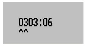
Use the plus and minus buttons to change the indicated part of the hobbs reading. Use the Select button to change from hour hundreds to hours to minutes. End the edit by pressing the Menu button.
