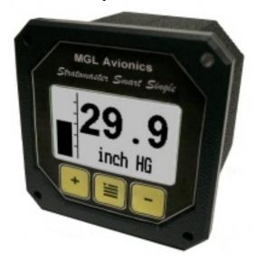
The MAP-1 is a 2.25" instrument which can measure pressures in the range from 0.25 bars (3.6 PSI) to 2.5 bars (36.2 PSI).
