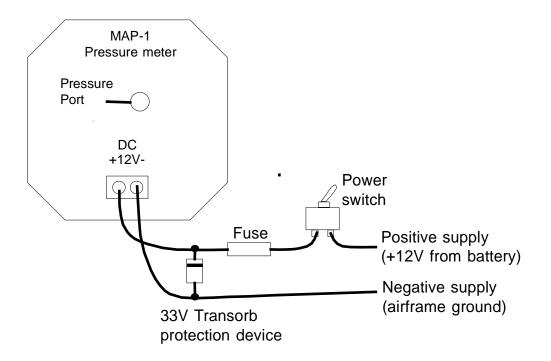
Connect the supply terminals to your aircrafts power supply (you need a dropping resistor or preregulator for 24/28V systems).
