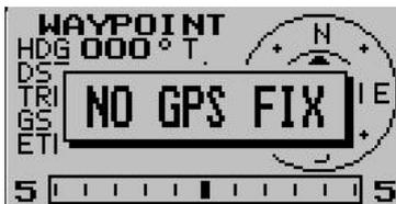
The GPS-1 will display a message box when trying to acquire a position fix. Once a 2D or 3D fix is achieved the message box will disappear.
