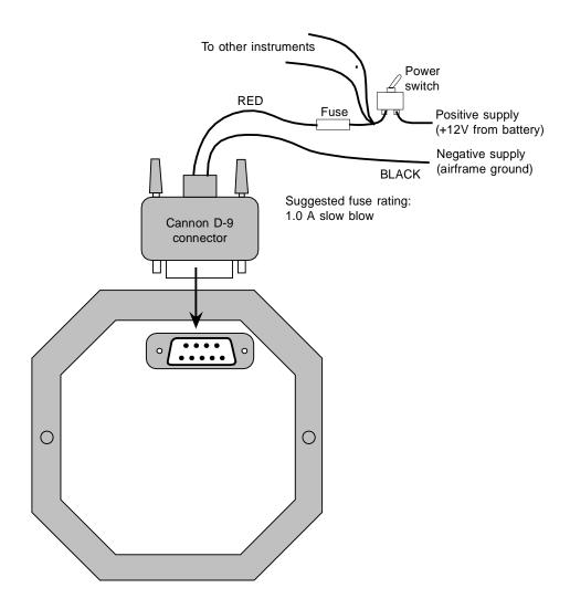
Connect the supply terminals to your aircrafts power supply (you need a dropping resistor or preregulator for 24/28V systems).
