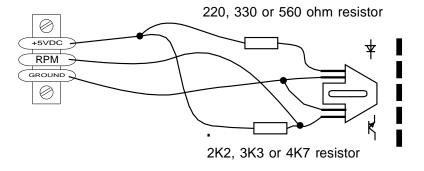
The optical reflective pickup can provide a simple means of contactless RPM sensing in difficult installations.
