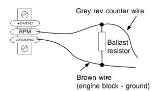
Note: On Rotax DCDI ignition systems it may be required to install a ballast resistor as shown. A typical value is 220 ohms. Many installations can omit this.
