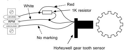
The gear tooth sensor is a popular pickup used on the pre-rotation gear of a gyro plane. (rotor speed indication)
