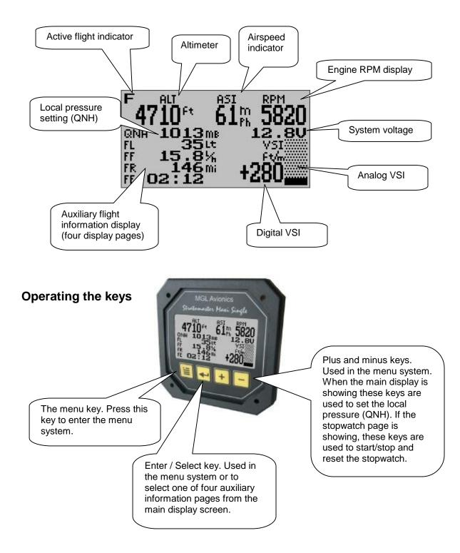
The bottom left section of the main display is arranged in four pages. Use the "Select" (Enter) key to page between these pages.
