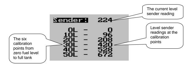
Performing the calibration procedure. Note: You start with an empty tank, you need a measuring jug or fueling device that has calibration marks and you need enough fuel to fully fill the tank.
