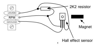
Typical hall effect sensor installation detects the passing of a magnet suitably fixed to prop flanges or shafts.
