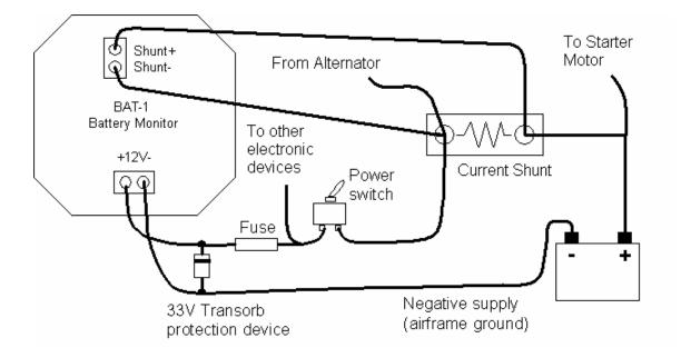
Connect the supply terminals to your aircrafts power supply (you need a dropping resistor or preregulator for 24/28V systems).Install suitable power supply protection if you have a supply that can contain large voltage transients such as can be created by starter motors and solenoids.
