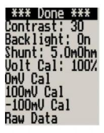
Press the Menu key to enter the menu. You can move forward and backwards in the menu by using the + and – keys. To change or select a menu item, move the highlight to the desired item and then press the Menu key. To end an edit or function, press the Menu key again.
