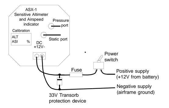
Installing the ASX-1 is quite straight forward.
