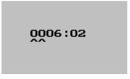
Use the plus and minus buttons to change the indicated part of the hobbs reading. Use the Menu button to change from hour hundreds to hours to minutes.
