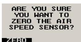
This setup allows your instrument to measure the zero airspeed reading of the airspeed sensor and set a calibration value internally for this. This is equivalent to some mechanical airspeed indicators that have an adjustment to set the needle to zero when the aircraft is not moving. You would use this function occasionally if you see an airspeed reading when
