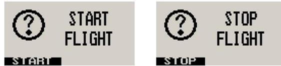
Press the F1 key during the normal display mode to manually start/stop a flight. This key is only active if the ASX-2 is setup to select the manual flight option under the log book setup menu.
