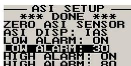
Enter the low airspeed set-point for when the alarm must activate. Any speed below this value will activate the alarm.
