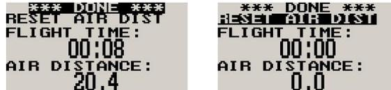
**Note:** The air distance trip counter measures distance flown through the air. This is not the same as distance flown over the ground unless you are flying at sea level at zero wind speed. The air distance shown is subject to under reading at altitude due to decreased air density.
