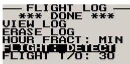
Select whether you want the ASX-2 to automatically detect a flight or whether the pilot must press the F1 key to start/stop a flight.
