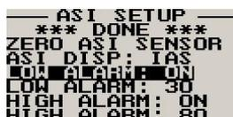
Select whether you want the low air speed alarm to be turned on or off. The low airspeed alarm is only activated once a flight has started.
