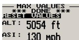
Move the highlight over this menu item and press the rotary button to reset the maximum altitude and airspeed values to the current values.
