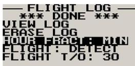
Select if you would like the hour to be displayed in decimal fractions (0-99) or minutes (0-59). This setting influences the current flight time display and the flight log.
