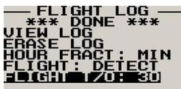
This menu item is only shown if the "detect" flight mode is selected. Enter the airspeed that you want a flight log entry to start.
