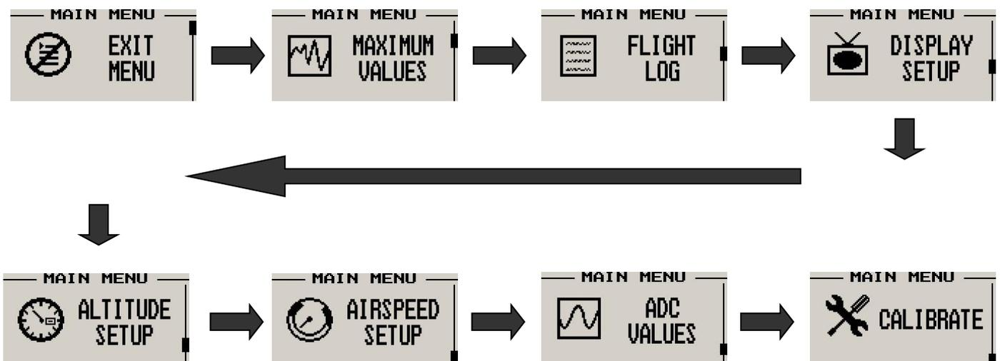
**Note:** (ADC Values and Calibrate Menus are only visible when powering up the unit and pressing the Rotary Control). The text "CALIBRATE" will appear on the intro screen when entering this mode.
