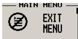
Pressing the rotary control on this menu item will cause the ASX-2 to exit the menu system. All changes made during navigation of menu system will be saved in non-volatile memory on exiting the menu system. If you remove power before exiting the menu the instrument will not save any changes.
