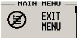
Press the rotary control on this menu item to exit the menu system. All changes made during navigation of the menu system will be saved in non-volatile memory on exiting the menu system. If you remove power before exiting the menu the instrument will not save any changes.
