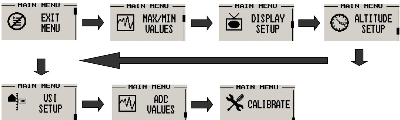
**Note:** (ADC Values and Calibrate Menus are only visible when powering up the unit and pressing the Rotary Control). The text “CALIBRATE” will appear on the intro screen when entering this mode.
