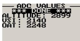
This menu displays the ADC values that have been read from the pressure sensors.
