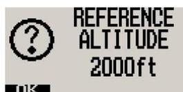
Enter the reference altitude you would like to use in relative mode. Use the rotary control to adjust the reference altitude. Press the F1/up key to accept.
