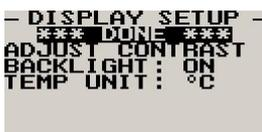
Move the highlight over this menu option and press the rotary button to return to the main menu.
