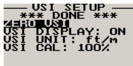
This function is used to set your VSI to read exactly 0ft/min. This is similar to setting the needle on a mechanical VSI to point to zero by turning the adjustment knob on such a VSI. The electronic VSI generally has much less drift compared to a mechanical VSI and this function will only be used very occasionally. Ensure that you perform this function when no pressure changes due to wind or other reasons are occurring.
