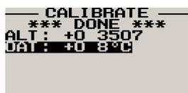
The ALT-3 is calibrated in degrees Celsius. The ALT-3 is calibrated at the factory using a precision laboratory thermometer. If recalibration is required then adjust the value using the up/down keys or the rotary control until the temperature matches the reference ambient temperature.
