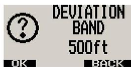
Adjust the deviation band above and below your reference altitude that is still acceptable to fly in. Any altitude outside this band will activate the alarm. Press the F1 key to accept, press the F2 button to return to the main display.
