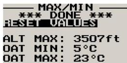
Move the highlight over this menu item and press the rotary button to reset the maximum altitude and airspeed values to the current values.
