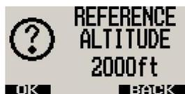
Adjust the reference altitude using the rotary control. This is the altitude that the pilot wants to maintain. Press the F1 key to accept, press the F2 key to return to the main display.
