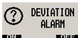
Select whether you want the altitude deviation feature enabled or not. Press the F1 key to enable the altitude deviation feature, press the F2 key to disable the altitude deviation feature.
