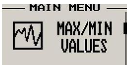
To avoid false recordings, the maximum values function is only activated 10 seconds after the instrument has powered up.
