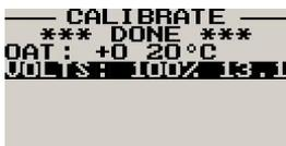
Adjust the voltage calibration constant until the reading matches your supply voltage measurement device (e.g. multimeter).
