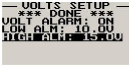
Enter the high voltage set-point for when the alarm must be activated. Any voltage above this value will activate the alarm.
