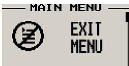
Pressing the rotary control on this menu item will cause the RTC-1 to exit the menu system. All changes made during navigation of the menu system will be saved in non-volatile memory on exiting the menu system. If you remove power before exiting the menu the instrument will not save any changes.
