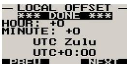
Select the main time zone that is to be displayed on the top section of the display. Normally this would be set to UTC.
