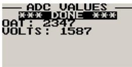
This menu displays the ADC value that has been read from the temperature sensor and voltage circuitry.
