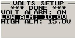
Enter the low voltage set-point for when the alarm must be activated. Any voltage below this value will activate the alarm.
