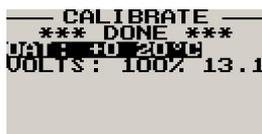
The RTC-1 is calibrated in degrees Celcius. The RTC-1 is calibrated at the factory using a precision laboratory thermometer. If recalibration is required then adjust the value using the up/down keys or the rotary control until the temperature matches the reference ambient temperature. The RTC-1 is now calibrated.
