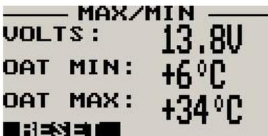
Press the F1 or F2 keys during the OAT/Voltage display to display the maximum/minimum values. Press the F1 key to reset the max/min values to the current values. To avoid false recordings, the maximum/minimum OAT function is only activated 10 seconds after the instrument has powered up.
