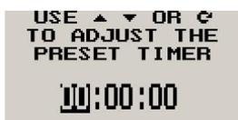
Enter the timer preset value. This is the value that is loaded into the timer when you perform a timer load. The timer counts down to zero when started, starting from this value. When zero is reached the alarm is activated.
