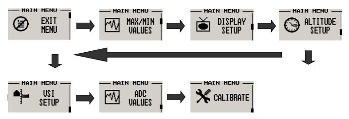
**Note:** (ADC Values and Calibrate Menus are only visible when powering up the unit and pressing the Rotary Control). The text "CALIBRATE" will appear on the intro screen when entering this mode.
