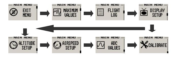
**Note:** (ADC Values and Calibrate Menus are only visible when powering up the unit and pressing the Rotary Control). The text "CALIBRATE" will appear on the intro screen when entering this mode.
