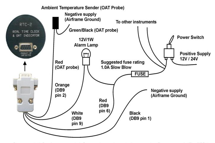
The use of an external 1A fuse is recommended. Connect the supply terminals to your aircrafts power supply. The RTC-2 can be used on both 12V and 24V without the use of any pre-regulators. Ensure that the supply voltage will not drop below 8V during operation as this may result in incorrect temperature readings.
