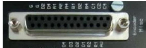
This is a DB-25 female connector. It contains the signals of the internal alticoder for use with a transponder. Note: Some newer type of transponders may no longer use these signals.
