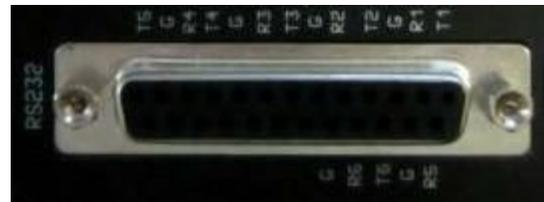
T1,T2,T3,T4,T5,T6 RS232 level compatible transmitters. These are connected to the receivers (RX) of the connected equipment.
