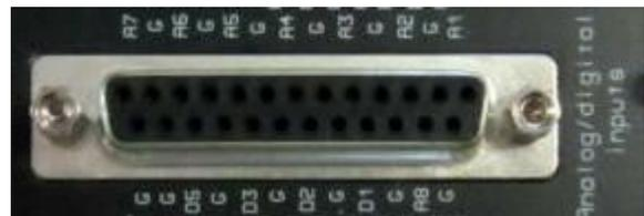
A1,A2,A3,A4,A5,A6,A7,A8 Analog and digital inputs. These eight inputs can be used as analog inputs with a measurement range from 0V to about 16V and a resolution of 4 millivolt (4096 quantization levels). They can be used as digital inputs based on a fixed threshold. Usage of these inputs is determined by the EFIS setup. Typical uses are flap and trim position measurement, gear status indication, etc.
