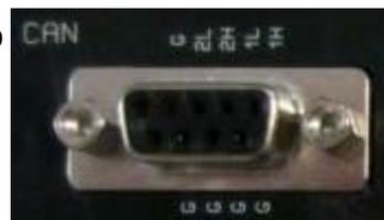
Note: Never connect the two CAN bus interfaces together – they must remain independent.
