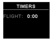
This display can be accessed by pressing the F2/Down button during the normal display mode.
