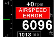
Airspeed sensor error. The instrument could have a faulty airspeed sensor in which case the instrument will then have to be returned to the factory. (Certain digital airspeed sensor models only)
