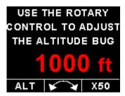
Press the F1/Up button during the altitude "TAPE" display to access the altitude bug setting screen. Press the F1/Up key to set the altitude bug to the current altitude or use the rotary control to adjust the altitude bug. Press the F2/Down key to change the increment / decrement unit to 50 or 500. Press the rotary control to exit and save.
