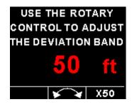
Use the rotary control to adjust the altitude deviation band. Press the F2/Down key to change the increment / decrement unit to 50 or 100. Press the rotary control to exit and save.
