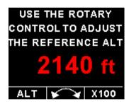
Press the F2/Down button during the Deviation Altitude display to access the altitude reference screen. Press the F1/UP key to set the reference altitude to the current altitude or use the rotary control to adjust the reference altitude. Press the F2/Down key to change the increment / decrement unit to 10 or 100. Press the rotary control to exit and save.
