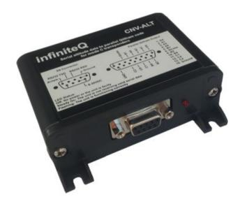
The CNV-ALT accepts RS232 serial data from a compatible MGL Avionics instrument and produces parallel Gillham codes in a format compatible with mode C transponders. The ALT-5 serial protocol must be set to MGL Avionics.
