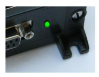
The green LED flashes at about 1Hz during operation. If the LED is steady "ON" there is a serious fault with the RDAC and it cannot operate. If the LED is "OFF" the RDAC is not being supplied with power or there is a serious fault with the RDAC. If the RDAC is connected to an EFIS the LED will perform a double flash to indicate that it is "seeing" the EFIS.
