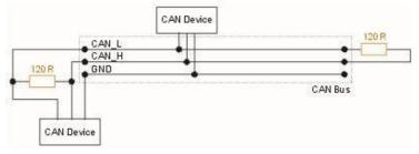
stubs to connect to equipment along the route. Never implement a CAN bus as a "star" or other wiring topology.
