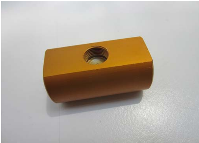
Image of the flow sensor body with sensor module removed
