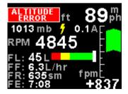
Altitude sensor error. The instrument could have a faulty altitude sensor in which case the instrument will then have to be returned to the factory.
