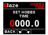
This function allows you to set the engine Hobbs meter to any value. Typically, you would use this function to set the Hobbs meter to the current known engine time. Use the rotary control to change the value. Press the rotary control to accept and exit the menu option. If the Hobbs code is set to another value beside zero, then the pilot will be prompted to enter the Hobbs access code before allowing him to change the Hobbs time. This feature is useful for charted and flying school planes.
