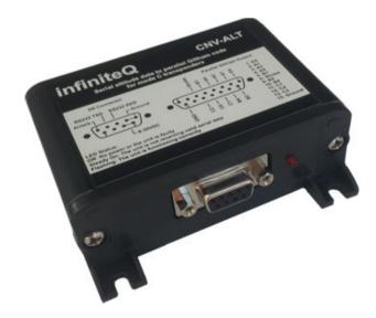
The CNV-ALT accepts RS232 serial data from a compatible MGL Avionics instrument and produces parallel Gillham codes in a format compatible with mode C transponders. The Flight-3 serial protocol must be set to MGL Avionics.
