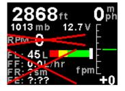
The red cross over the displays means that the FLIGHT-3 has lost communications with the external RDAC unit. Check the wiring between the FLIGHT-3 instrument and the RDAC unit. This error message is only shown when the external RDAC is selected as the data source.
