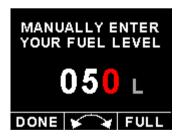
Press the F1 key during the main display screen to manually enter your current fuel level after fueling or defueling your aircraft. This function is only available if you have selected fuel level is calculated from fuel flow. Press the F2 key as a "quick fill button" to the full level.
