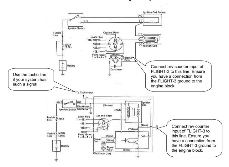
Electronic ignition system with conventional ignition coil
