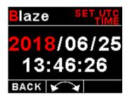
This function is used to set the internal real time clock. The time to be entered must be UTC in order for the system to operate correctly. Do not enter local time (unless it is the same as UTC).
