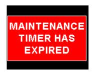
A maximum of 999 hours can be entered as a maintenance interval. A reminder message will appear on startup when zero hours are remaining. The reminder message will disappear after the pilot presses any key. Engine running time for the purpose of the maintenance timer is defined as the run time where the engine RPM is greater than the "HOBBS RPM" value as set in the "TIMERS SETUP".
