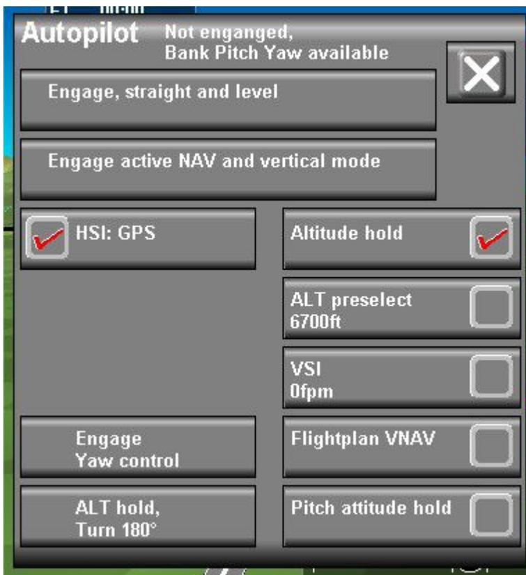
If the autopilot is enabled and configured, select the autopilot control dialog using either the “AP” button or tap on the autopilot status display.
