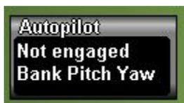
Pressing “Engage, straight and level” will engage the autopilot in current heading and altitude hold mode. Heading is derived from GPS heading corrected for local variation to obtain magnetic heading. This means that heading is independent of your compass installation. Altitude is derived from your altimeter and thus responds to local pressure settings. Your altitude bug is set to the nearest 50 ft boundary.
