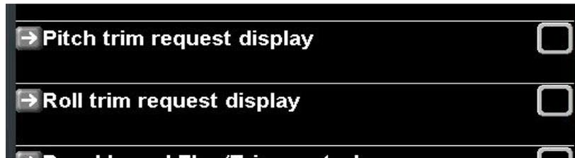
Your screen design must have the required visual indicators placed (standard screens have them by default). These are invisible until stick forces are measured that require an adjustment of trim. Note that to be able to measure stick forces servo torque setting must be 80% or less. It is possible to go as much as 85% but with reduced sensitivity.
