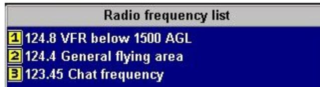
Frequencies and description are stored in a simple text file that you can create yourself (using Notepad or similar) with a filename of "radio.txt". Please use a simple text editor to create a normal ASCII text file. Do not use files created by Word processing applications unless they can export to a simple text file.
