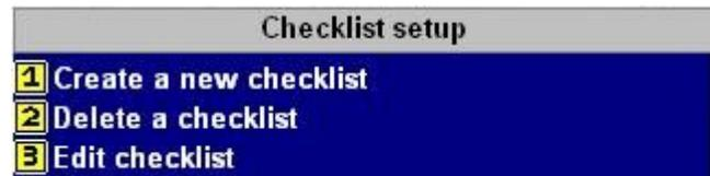
Checklists can be activated and deactivated from any main display screen by selecting “Shift-Check”.
