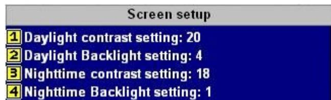
Backlight level settings have a significant effect on power consumption of your instrument. Do not use a backlight setting higher than what is required in your aircraft for best display quality.
