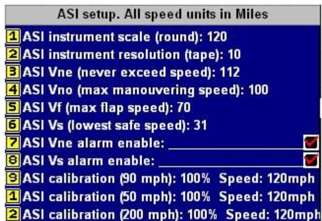
Example: Your 50 mph factor is 120%, your 90 mph is 100% and your 200 mph is 90%. With this setting, your airspeed will readout according to factory calibration at 90 mph, it will read 5% less at 145mph, 10% less at 200 mph and 15% less at 255mph. At 70mph airspeed will read 10% higher, at 50mph 20% higher
