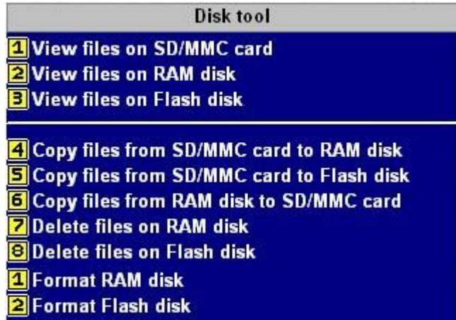
You can format both RAM drive and Flash drive if for some reason they have been corrupted. After formatting the Flash drive you need to reinstall screen files, waypoint and abbreviated airport information file.
