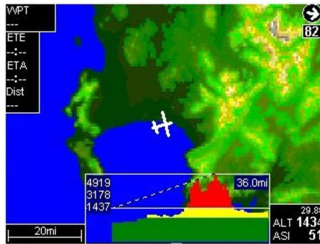
In the absence of raster image maps, the EFIS can use terrain data to create topographical maps using shades of color to indicate ground elevation. A typical image this creates is shown above of the Cape Town area, where your EFIS instrument has been developed. No particular setup is required. If your SD does not contain any raster map data for the area under consideration but terrain data is available, the terrain data will be used automatically.
