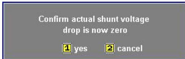
This sets the zero current calibration point. This is stored in the current monitoring device, not in your EFIS.
