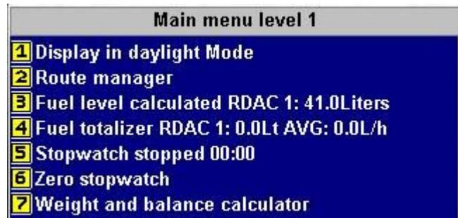
The Weight and Balance display allows you to enter weights that do not change in flight, for example passenger and baggage as well as fuel tanks related directly to the 6 possible fuel tanks that your EFIS can monitor (4 physical tanks and 2 calculated tanks if you have two RDACs connected). In case of these fuel tanks, weights and balance will be calculated using current fuel levels, zero fuel level (in RED color) and full fuel level (in GREEN color).
