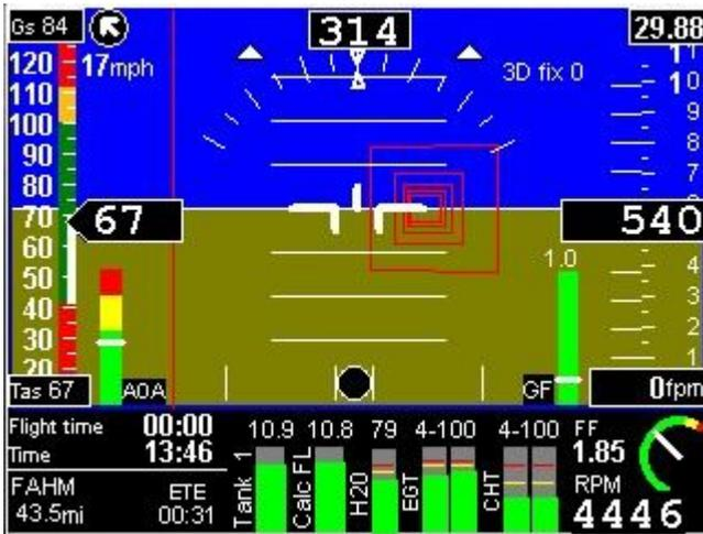
Should your heading be more than +/-90 degrees from the desired heading to reach the next waypoint, the highway is drawn in red as shown in the picture on the left. You need to reverse course as you are flying away from your target.
