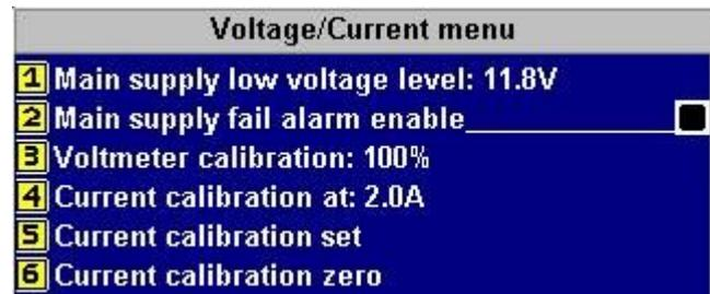
Main supply low voltage level specifies the voltage below which the “Low voltage alarm” is activated. Note that you still need to enable this alarm in the “Alarm setup and routing” if you want to use this alarm.
