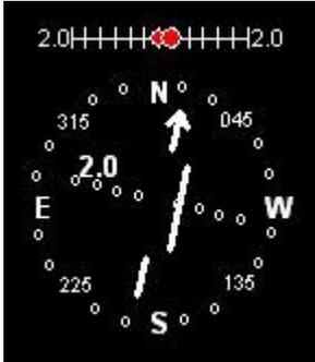
This image shows the two types of GPS based CDI displays supported with the current version of the EFIS. The top display is a true CDI which in this case is telling you that you are about 2 miles to the left of the desired track and you should steer right to intercept the track.
