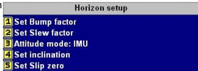
Set slip zero – this function allows you to set your slip indicator to exactly zero even if your aircraft tends to fly slightly wing down. The procedure is to place the aircraft in a stable, straight and level attitude during calm flight conditions and then select this function.
