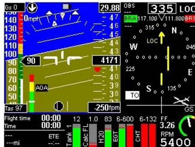
The above screen shows the active NAV channel tuned to a localizer station. In this case we are to the left of the runway centerline and should adjust to the right to intercept. Note the third form of available glide slope indication. This display has the aircraft symbol move from the top right (very high) to the bottom left (very low) of the indicator. If you keep the aircraft exactly centered on the cross hair, you will be exactly on the glide slope.
