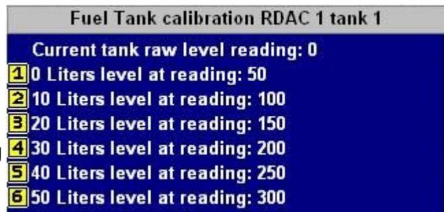
at zero volts, while a reading of 4095 is equivalent to 5V. Important is that the reading changes with your fuel level **in a repeatable and reliable way**. The EFIS does not mind if the reading increases or decreases with fuel level, as long as it does so in a meaningful way.
