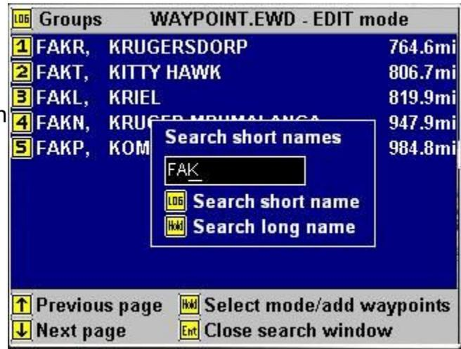
Tip: Waypoints created on the fly using the “mark” function are stored in order of creation in the route file “markers.ert” located on your RAM drive. You can add waypoints from the markers route file (or any other route file) by selecting “pick from a route” and then selecting the desired route name.
