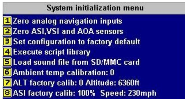
You will use this function if you find that your airspeed indicator is showing a small, permanent reading or your VSI is showing a climb or sink when ambient pressure is constant. We find the sensors seldom drift by much during aging but it is usually a good idea to perform this function once a year or when the need arises.
