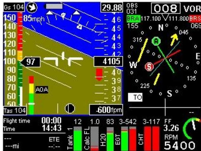
The above image shows a typical implemented VOR display, fully active. Note that a thin, light blue line is drawn as well, this is the current ground track as indicated by the GPS. It shows quite a deviation from the heading which can be expected noting that we have a very strong 85 mph wind blowing from the left in this example.
