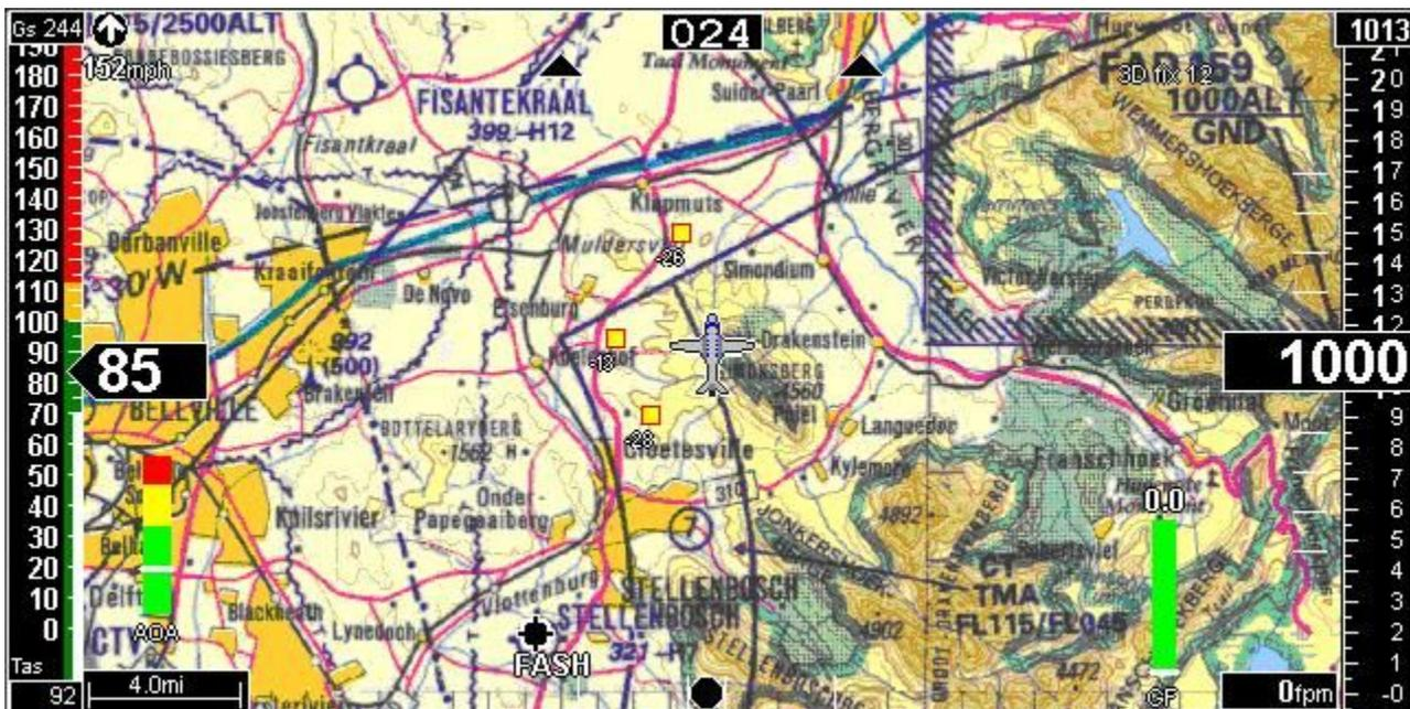
A typical raster map image. The source of the image is a scanned aviation chart that has been converted to Enigma raster map format by the free Enigma Mapmaker program (available for download from the MGL Avionics website).
