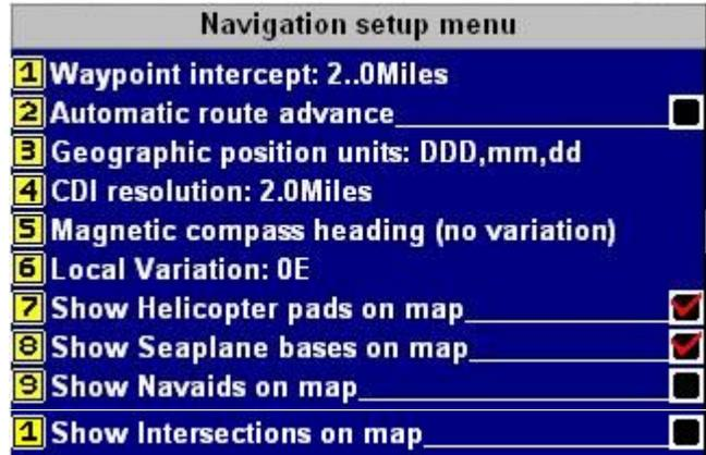
Magnetic variation for your location is automatically calculated for your current location using a comprehensive model of the Earth magnetic field and how it changes with time. For magnetic variation to be correct, it is important that you enter the correct time and date into your EFIS (time and date setup).
