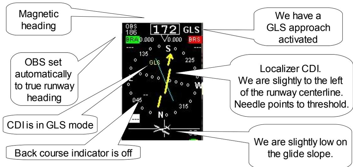
The above display is taken from an approach onto Runway 19. The actual magnetic heading is 186 degrees. The OBS is set automatically to this when you select the GLS approach. The true heading in the airport database for this runway is 162 degrees and the variation is 24 degrees west which gives 184 magnetic. The runway threshold is also set as “goto waypoint”
