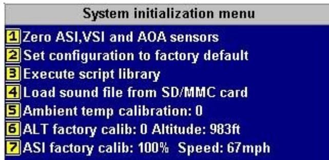
Executing a script file can be used to setup your EFIS from a preprepared script created using the EFIS Screen Designer and Simulator program. This function is also available from the “Install Tasks” menu. Scripts can be used to easily copy an entire setup, including screen designs to an EFIS instrument.
