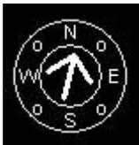
This image shows an alternative navigation instrument created with two components, the small compass rose and a heading error set to show “track error”.
