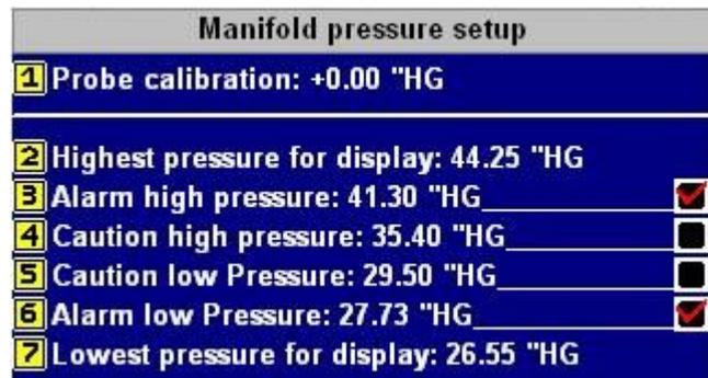
display). Compare the MAP reading with the barometer and adjust the MAP until it reads exactly the same pressure as the barometer which on EFIS shows actual ambient pressure.
