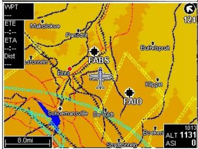
Note: You change between raster and vector modes by using SHIFT+5 from any main screen. First press “SHIFT” and then “5” (map).
