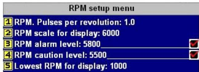
well to cater for unusual engines such as three cylinder engines.
