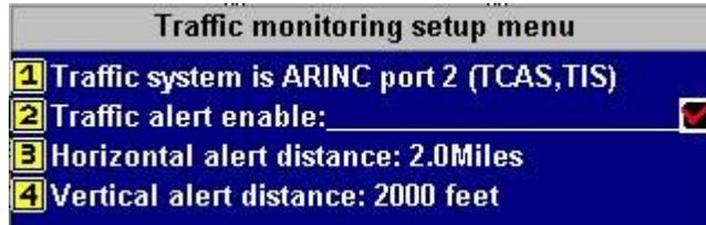
Using the provided menu in the System Setup menu, select the desired source for traffic monitoring. You can select multiple sources such as TCAS/TIS and FLARM or TCAS/TIS and PCAS.
