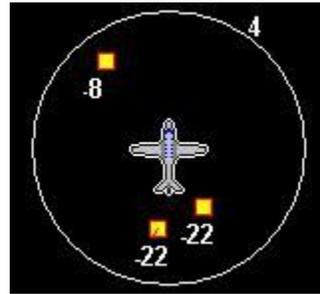
Traffic is displayed as a small yellow square with red border and can be trailed by a red flight path if previous history of this intruder is available. Underneath the intruder the relative altitude is displayed in steps of 100 ft. Negative values mean the intruder is below your altitude while positive numbers show intruders above your flight altitude.
