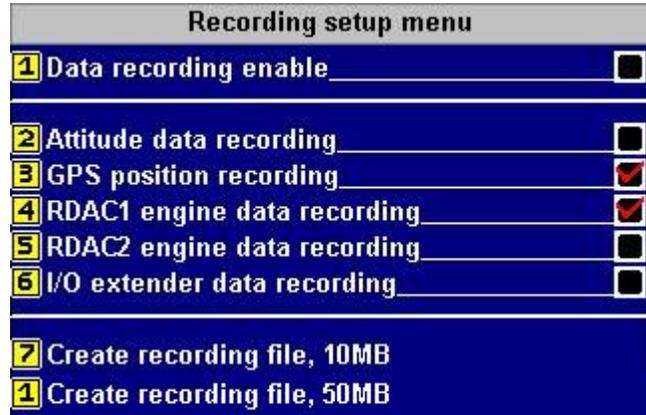
Alternatively you can create two default sizes of recording file using your EFIS. As a rule of thumb, you can work on about 1 MB per hour for an average system setup. Writing the recording file onto the SD may take some time to complete depending on the maximum write speed of your SD card. Make sure the cards “write protect” tab is in the “off” position. No writing to card is possible if the “write protect is active”.
