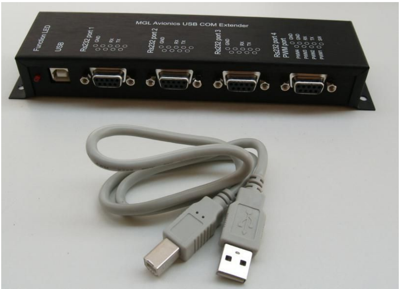
MGL Avionics USB COM Extender and autopilot servo interface
